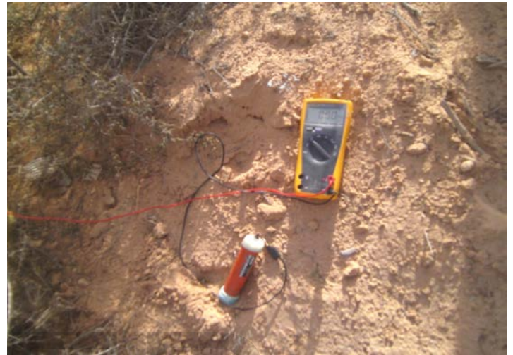
Figure 2.4- Reference Electrode with digital device voltmeter
