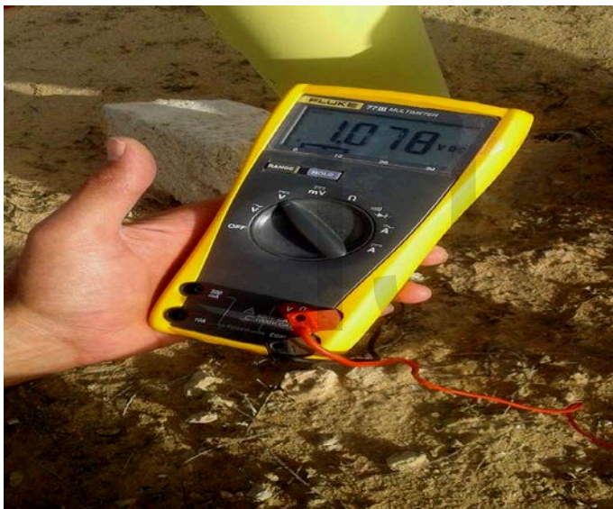
Figure 2.6- Pipe to soil potential actual measurement
